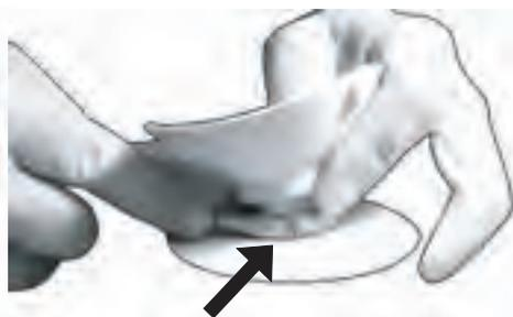
2) With a flat screwdriver, compress the Step Cup™ mushroom ring while pushing it into the hole.
