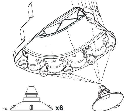
1) Insert half of the Step Cup™ mushroom in the hole, at a 45 degree angle.
