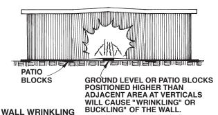
Prevent wrinkling of the pool wall during installation by checking and rechecking the levelness of the ground and patio blocks (Optional) at each vertical (Steps 2 and 10). If one patio block is higher than those positioned at each side, wrinkling of the wall will occur when wall is installed.
