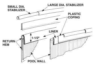
Make a return hem as illustrated. DO NOT cut off excess liner material as the liner will "Slip" from under the plastic coping, causing liner to fall back into the pool. **Smooth liner against wall and secure to top of wall with plastic coping.** Place stabilizer rails over coping, alternately telescoping small diameter into large diameter about 6 inches as before. One large diameter stabilizer rail fits between each pair of side supports. They DO NOT telescope.
