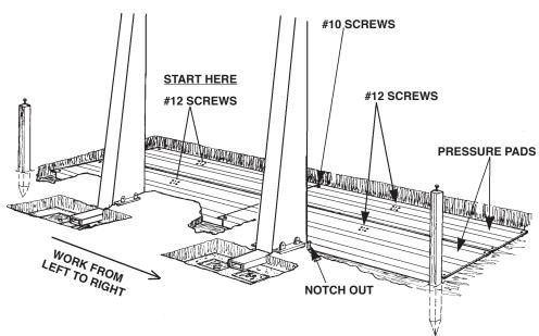
Keep the tops of the ground supports free of dirt. Working from left to right, assemble a set of pressure pads to each ground support using six (6)  $\#12 \times 3/4$ " screws as shown in Fig. A, (refer to your parts list as needed). Tighten screws firmly. Assemble each pressure pad set to its adjacent set using four (4)  $\#10 \times 1/2$ " screws. DO NOT OMIT ANY SCREWS.
