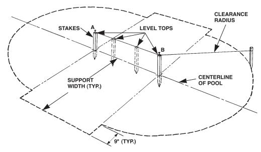
Refer to Pool Layout Dimensions for your pool size. Locate stakes A and B. Level tops with long 2" x 4" board and carpenter's level. For longer pools, intermediate stakes leveled between stakes A and B may be necessary. Layout clearances as shown.
