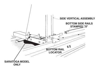
Loosely assemble bottom rails (stamped "S"), groove up, between verticals with bottom rail locators. Secure bottom rail locators to side verticals with screws. NOTE: Be sure to use the top set of holes in the side verticals when assembling the bottom rail locators.
