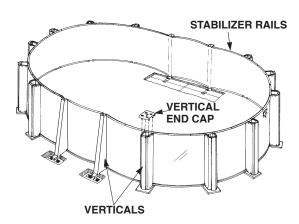
Carefully follow the detail for your pool shown in either Figs. B,C, D, E or F to assemble the verticals and vertical end caps to pool. Use all necessary hardware. Refer to your pool parts list.
