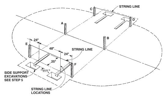
Locate Stakes C, D, E and F from your pool layout. Attach strings between C and D, then E and F. The first side support excavation is positioned 24" from the center of either stake to the center of the excavation. Other side support excavations are 48" center to center.
