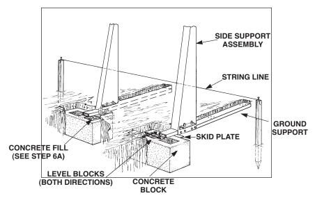
Remove string line. Place concrete blocks into the excavations as shown. **NOTE: The thicker wall side of the cement blocks must face up.** Level the blocks in both directions. Place the assembled side supports into each trench with skid plate resting firmly against the face of the concrete blocks. Check each ground support for level (refer to Step 6A).
