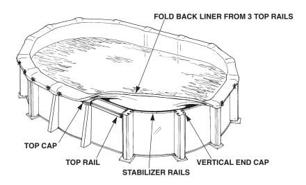
With the help of two or three people, raise and hold the liner up from any three top rail sections. Remove four top caps, three top rails, two vertical end caps and stabilizer rails. REMEMBER, NEVER ALLOW LINER TO FALL BACK INTO POOL.
