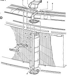
Three piece vertical assembly. Slide the center section (with two holes at top) down the grooves formed on each side section. Special Note: Special top connector assembly. After completing Step 16, attach vertical skirt to vertical, then attach top connector and decorative strip. Refer to your pools parts list and this guide for parts identification.
