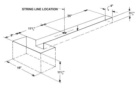
Carefully dig out the side support trenches following the dimensions above. It is very important that the trench walls remain firm and undisturbed during and after excavation. **DO NOT** over-excavate with the thought of back-filling later because the side supports will move when pool is filled, and pool failure may result.
