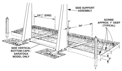
Dig out a trench to the dimensions shown above, grading to the ground support. Use a large screwdriver to scribe grooves (approximately 1" deeper) down each side and center of the trench to accomodate the pressure pads' flanges. Remove the excess dirt accumulated from scribing.
