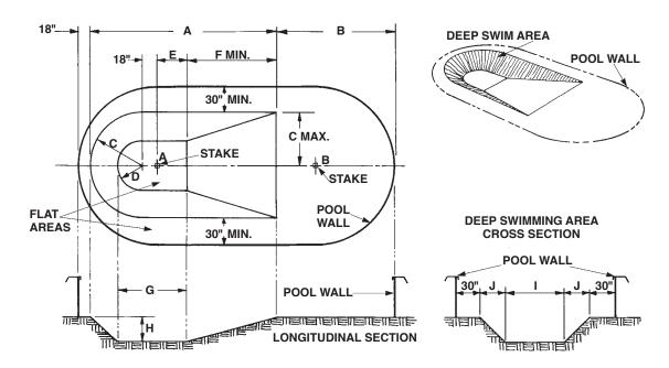
**ONLY 20 MIL. LINERS OR THICKER -** You may decide to excavate a deep swimming area as shown above. **The Deep Swimming Area is for underwater swimming only, NO DIVING, NO JUMPING.** To excavate the deep swimming area, use the layout illustrations above, along with the measurements from the chart for your size pool.
