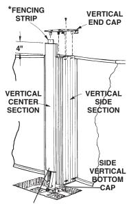
NOTE: SIDE VERTICAL CENTER SECTIONS ARE NOTCHED FOR **CLEARANCE OVER THE SIDE SUPPORTS**
