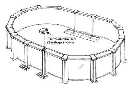
Attach all hardware and brackets and top connector as shown in detail of your pool. Refer to Figure B, C, D, E, or F.
