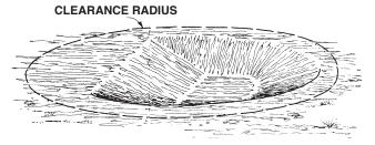
You may decide to excavate a deep swimming area as shown. The Deep Swimming Area is for underwater swimming only, NO DIVING, NO JUMPING. To excavate the deep swimming area, use the illustration shown, along with the measurements from the chart for your size pool diameter.
