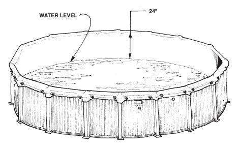
Continue filling pool. **Never allow liner to fall back into pool.** Water between the liner and wall can cause pool failure. When pool has approximately 24 inches of water, stop filling. Do not resume until Steps 18, 19 and 20 are completed. **CAUTION:** Do not cut any openings into liner at this time.
