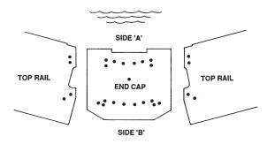
Each pool size has a specific hole pattern for mounting the top rails to the vertical end caps. Use the figure that matches your pool series, size, and the accompanying chart to locate the correct mounting holes.
