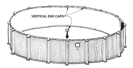
Carefully follow Figures A, B, C, D, or E to attach vertical end caps to verticals. Check pool for roundness. Check straightness of verticals using level tool.
