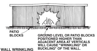
Prevent wrinkling of the pool wall during installation by checking and rechecking the levelness of the ground and patio blocks (Optional) at each vertical (Step 3). If one patio block is higher than those positioned at each side, wrinkling of the wall will occur when wall is installed.
