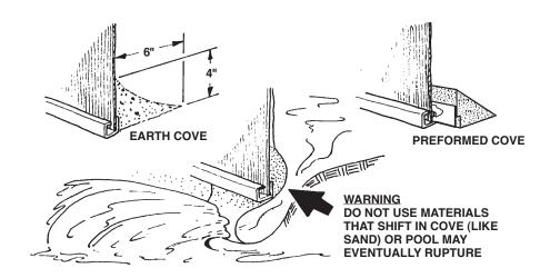
**Important Step:** The cove is a vital structural element that prevents water pressure from forcing the pool liner out under the bottom rail. The manufacturer will not assume responsibility should the cove be omitted.
