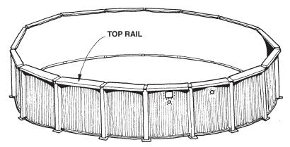
Attach all top rails using the chart from Step 9 to determine proper holes for attachment. At this time it is extremely important to check the framework to assure level installation. Place the level on each top rail, working gradually around pool, to assure framework is on flat ground with opposite sides no more than 1 inch out of level. **Remember: Always remove dirt to adjust framework - never fill in!**
