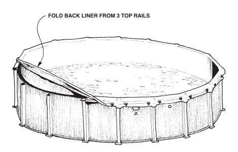
With the help of two or three people, raise and hold the liner up from any three top rail sections. Remove the attaching hardware at the top rail connectors, three top rails, three vertical end caps and stabilizer rails. REMEMBER, NEVER ALLOW LINER TO FALL BACK INTO POOL.
