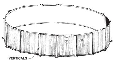
Carefully follow the details shown in Fig.s A, B, C, D, or E to assemble verticals to the pool wall. Refer to your pool parts list for parts identification and use all necessary hardware. Check pool for roundness by measuring across the pool from side to side. Pool diameter should be the same from point to point.
